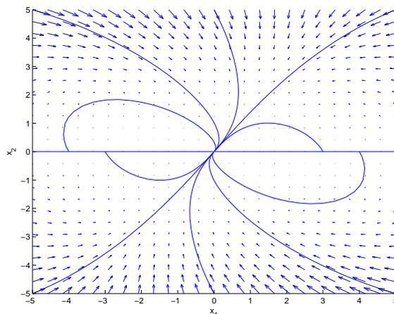
FIGURE 1. An a.g.s. system without local asymptotical stability. The system's equations are  $\dot{x}_1 = x_2 \cdot (-6x_1x_2 - x_1^2 + 2x_2^2)$ ,  $\dot{x}_2 = x_2 \cdot (2.229x_1^2 - 4.8553x_2^2)$  [6].
